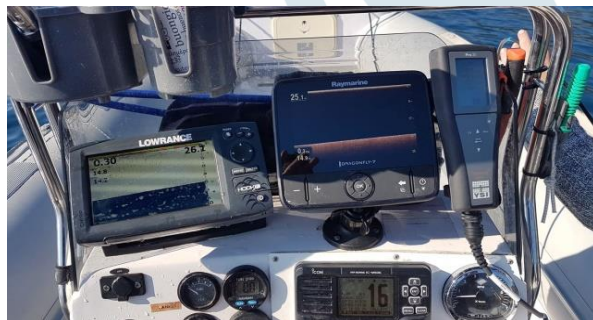
Below: the instrument used for collecting physicochemical parameters of the seawater
